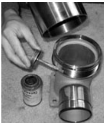
Figure 7-43 – Tighten Shell
