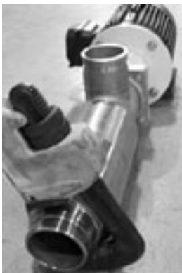
Figure 7-26 – Loosen Outlet Nozzle
