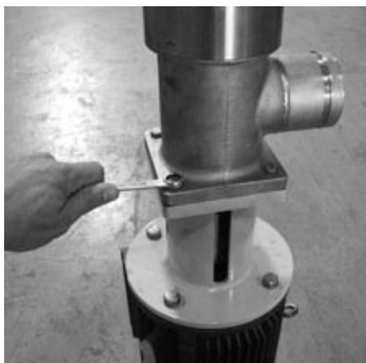
Figure 7-25 – Final Step: Tighten Inlet to Bell Housing
