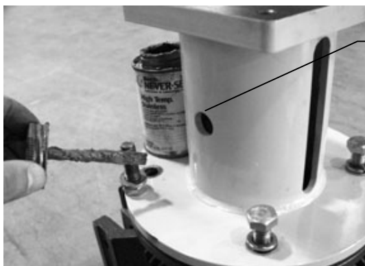
Figure 7-29 - Install Coupling and Bell Housing
