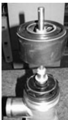
Figure 7-28 – Remove Shell and Stages
