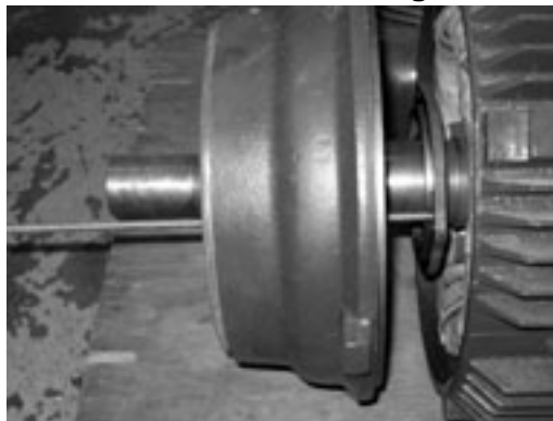
Figure 7-51 – Use All-thread to Align Retainer Plate
