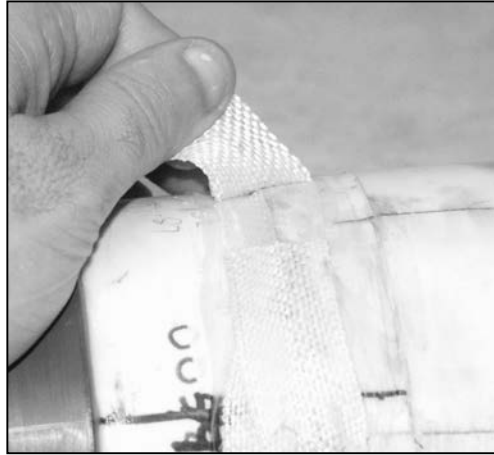
Figure 8-18 Remove Fiber Glass Tape
