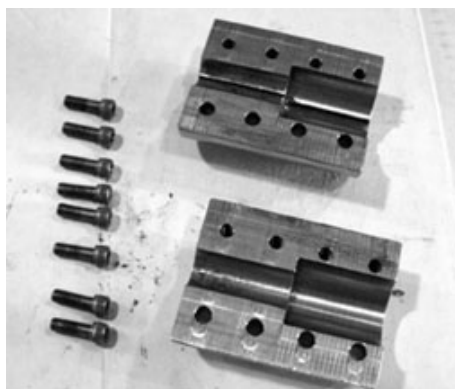
Figure 7-10 - Disassemble Coupling and Clean Components
