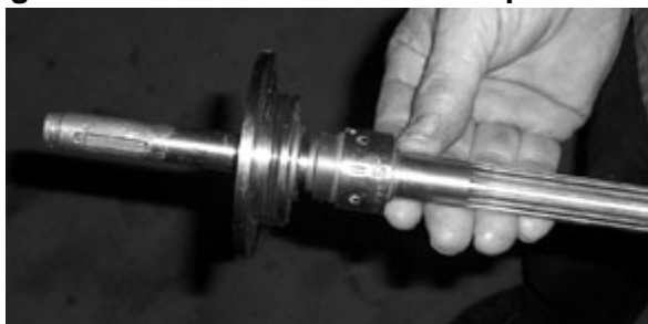
Figure 7-30 – Install seal and seal plate onto shaft
