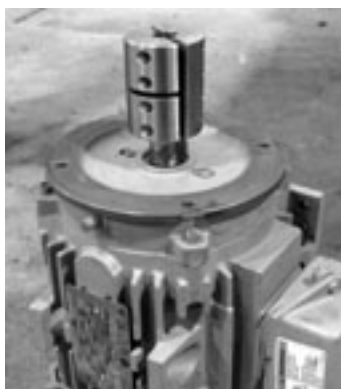
Figure 7-11 – Install Coupling and Bell Housing onto Motor
