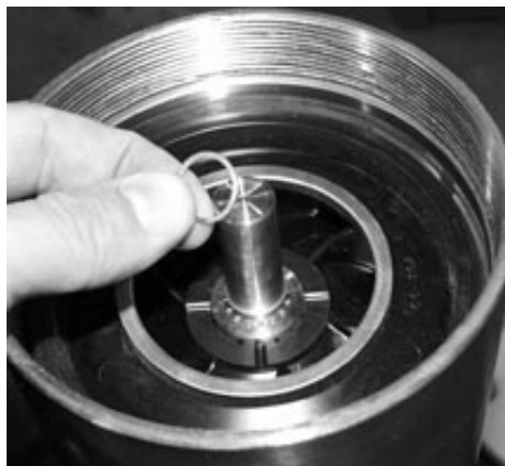
Figure 7-41 - Install Snap Ring, 8500-, 1250-Series
