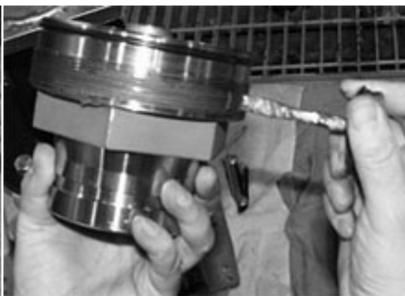
Figure 7-44 – Tighten Outlet Nozzle
