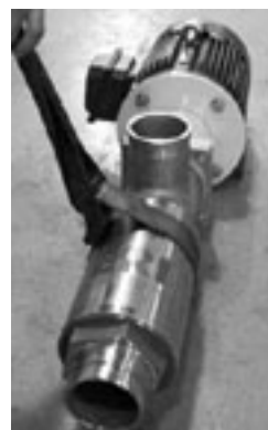
Figure 7-27 – Loosen Shell
