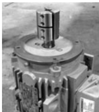
Figure 7-29 - Install Coupling and Bell Housing
