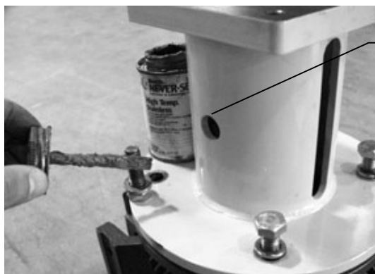
Figure 7-11 – Install Coupling and Bell Housing onto Motor
