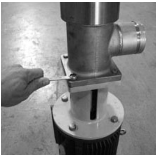
Figure 7-4 - Remove Pump from Bell Housing
