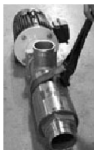
Figure 7-43 – Tighten Shell
