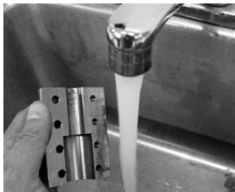
Figure 7-10 - Disassemble Coupling and Clean Components
