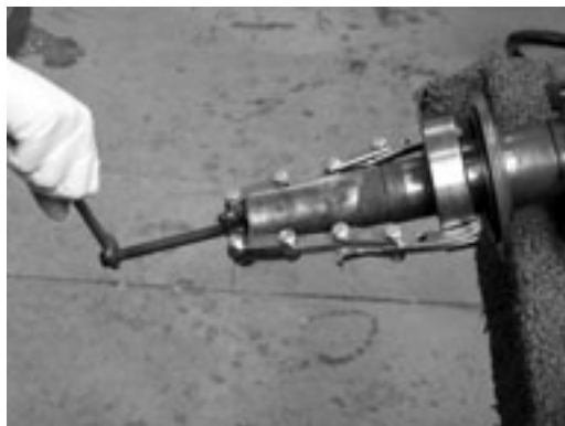
Figure 7-49 – Pull Bearing with Bearing Puller
