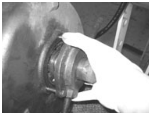
Figure 7-45 – Remove Bearing Lubrication Covers
