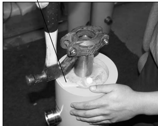
Figure 8-3 Remove Access Cover Position II
