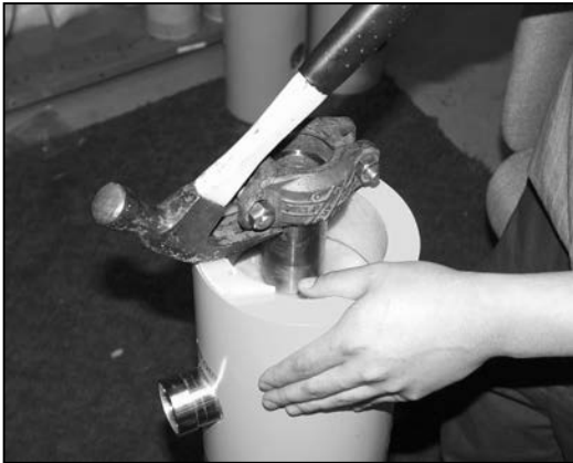
Figure 8-2 Remove Access Cover Position I
