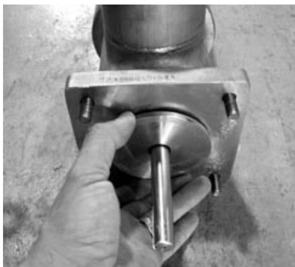
Figure 7-5 - Remove Seal Plate from Inlet
