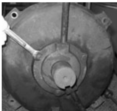
Figure 7-45 – Remove Bearing Lubrication Covers
