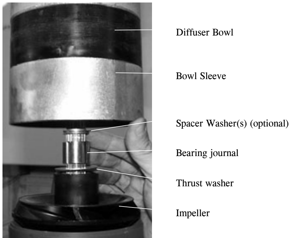
Figure 7-39 - Complete Stage Assembly for 2400-Series Pumps
