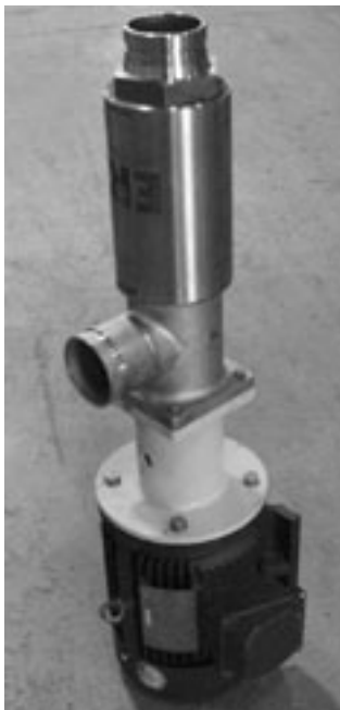
Figure 7-4 - Remove Pump from Bell Housing
