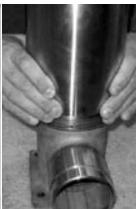
Figure 7-43 – Tighten Shell
