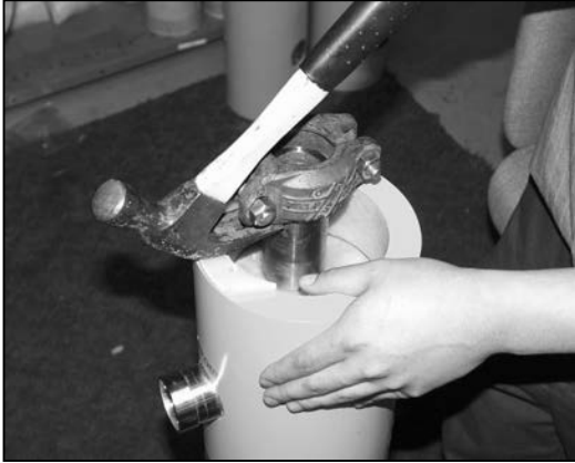
Figure 8-13 Remove Access Cover Position I
