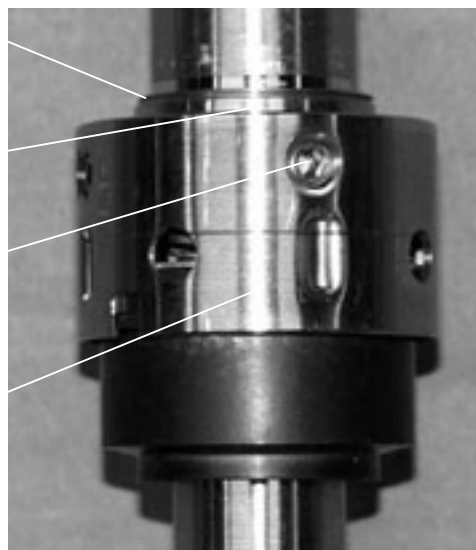
Figure 7-13 - Primary Seal Assembly
