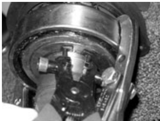
Figure 7-48 – Remove Bearing Retaining Ring
