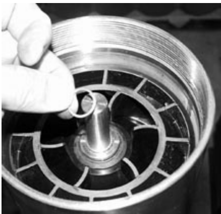
Figure 7-40 - Install Snap Ring, 2400-Series
